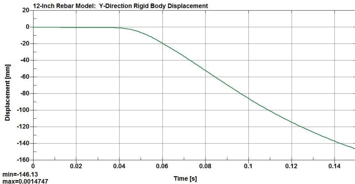
Figure 5.1.5: 12-Inch Rebar Model (12" Run 6): Rigid Body Vertical Displacement of the slope face shelter top with no filter applied.
