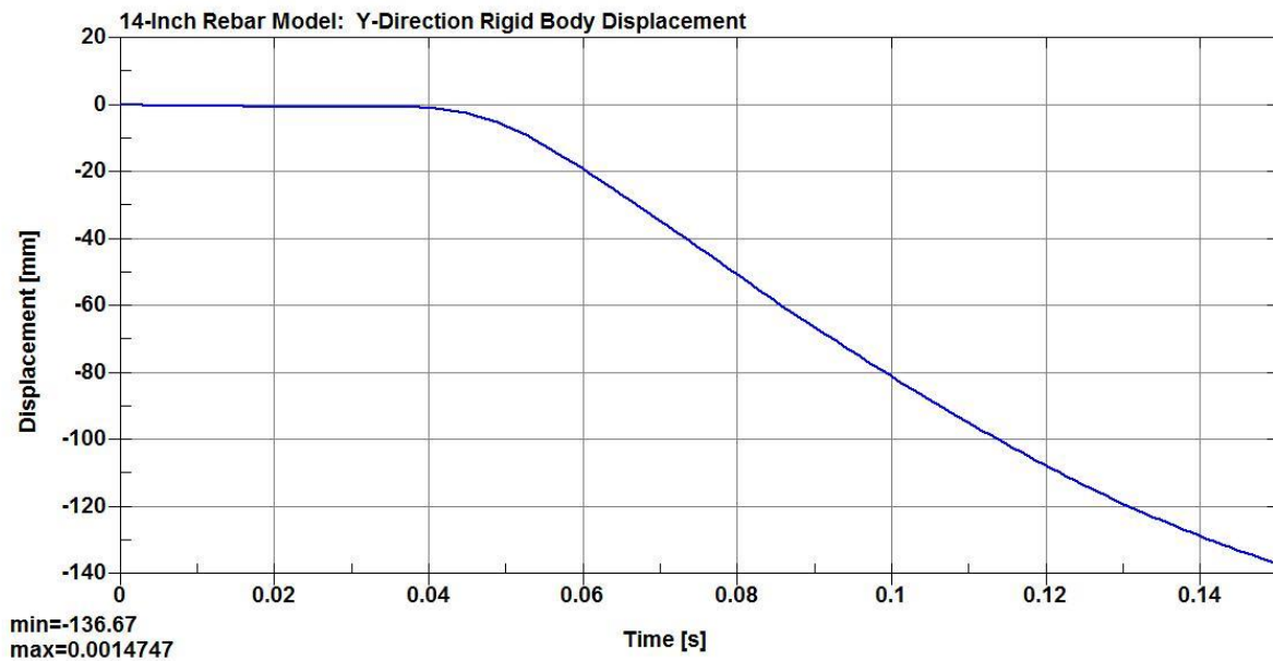
Figure 5.2.4: 14-Inch Rebar Model (14" Run 3): Rigid Body Vertical Displacement of the slope face shelter top with no filter applied.
