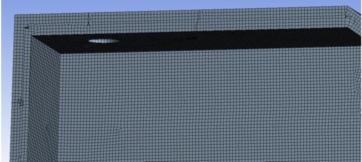
Figure 3.3.1: Cross-sectional view of the meshed lattice, positioned at the inside corner of the roof of the Slope face shelter . Note that it is predominantly hexahedral with few lattice imperfections.
